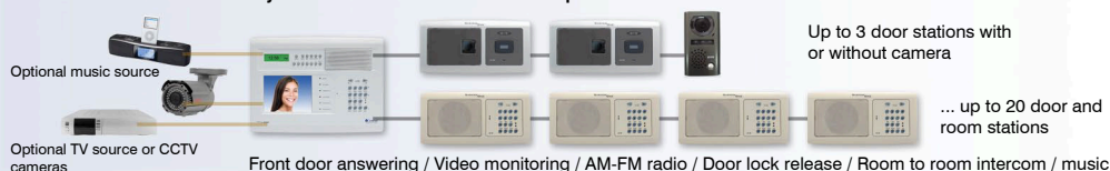
Front Door Stations with video options available in Bronze and Silver. Recessed door stations & room stations, Fascia: 265(w) x 130(h) Recess: 205(w) x 95(h) x 30(d)mm Surface mount Metal Door Stn 100(w) x 173(h) x 25(d) with flush option
